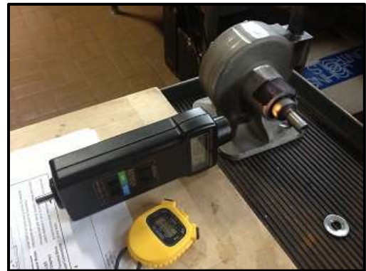
Figure 2: Optical tachometer and stopwatch positioned in the same video shot to enable video capture of turbine spindle experimental rotational velocity time histories for data analysis.
