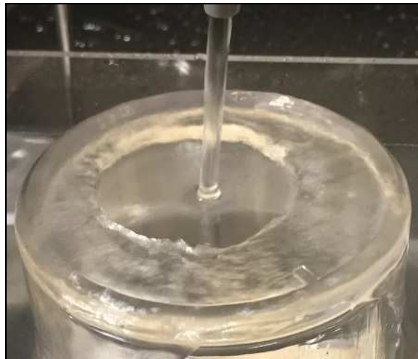
Figure 1. A representative circular hydraulic jump formed when a vertical water jet impinges on a flat horizontal surface.
