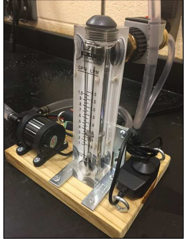
Figure 3. The hydraulic jump pump and flow rate component includes an aquarium pump, which moves fluid through the experiment and is speed-controlled by Pulse Width Modulation (PWM).
