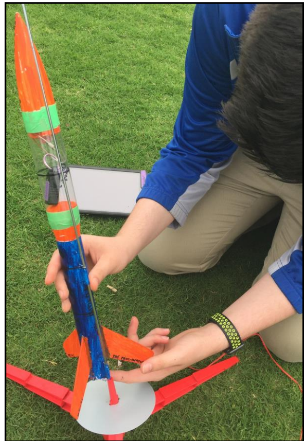
Figure 4: This student's rocket, loaded with a C6-5 motor is being prepared for launch. The AltimeterThree is visible, secured in the payload section, and the nosecone is taped to prevent it from falling off during flight and recovery.
