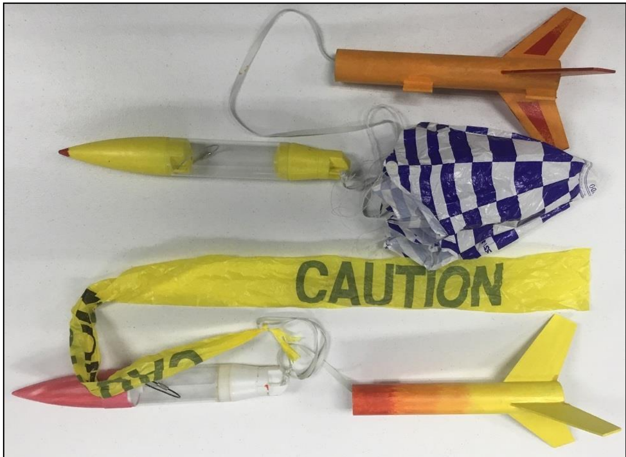
Figure 3: An unmodified Estes LoadStar II rocket (Top) was built by the instructor to establish an altitude performance baseline. Here, it is compared against a student-modified rocket. In this case, the student realized weight from the original rocket's parachute recovery system could be reduced by switching to streamer recovery, which facilitated safe return of the rocket but with less initial takeoff weight.
