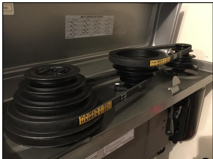
Figure 6: Drill press bit rotation rate is set by adjusting locations of a pair of belts between pulleys of different diameters mounted on two spindles inside the machine’s case. The STEM class’s drill press was capable of 16 unique speeds over a range from 200 to 3630 rpms.
