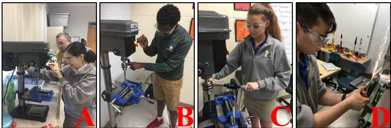
Figure 3: Under instructor supervision students (A) drilled out the nylon bolt, (B) drilled a hole through the aluminum blank, (C) tapped the blank with 1/2"-13 threads, and (D) de-burred and finished the machined blank either using sandpaper or a belt sander.
