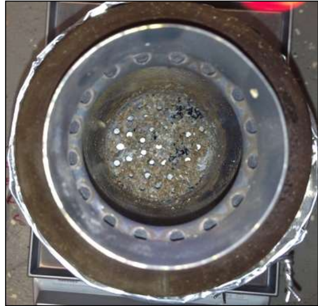
Figure 5: The gasifier's inner container, where fuel is retained, was imaged after a burn sequence to show the trace amount of ash remaining.
