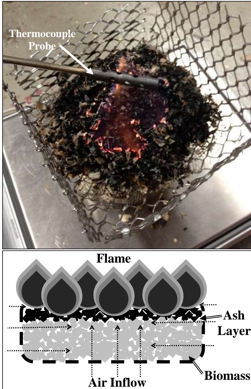
Figure 2: (Top) An open basket made from scavenged metal mesh holds wood chips undergoing conventional combustion. (Bottom) A schematic representation of the direct combustion burner shows locations of biomass fuel, airflow paths, and the ash formed at the combustion front.
