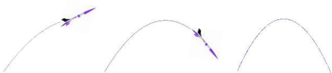
Figure 3: Typical oblique rocket launches result in classical parabolic flight trajectories.
