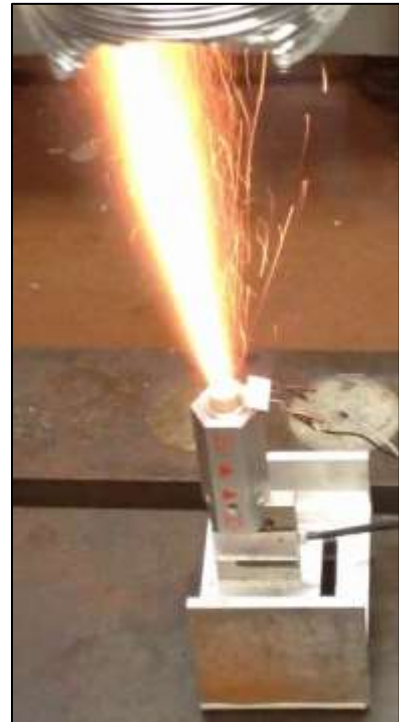
Figure 8: An Estes A8-3 model rocket engine is tested on the motor thrust apparatus.
