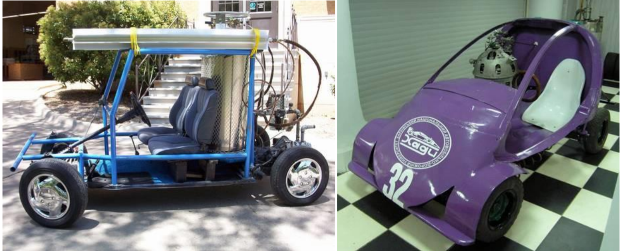
Figure 1. Experimental Cryogenic Vehicles Operating on LN 2 : UNT (left) and KNAHU (right).
