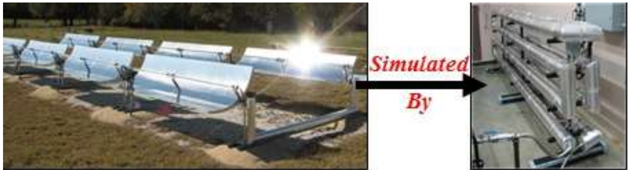
Figure 1. Performance of parabolic solar collector troughs was mimicked by a well-insulated simulator.
