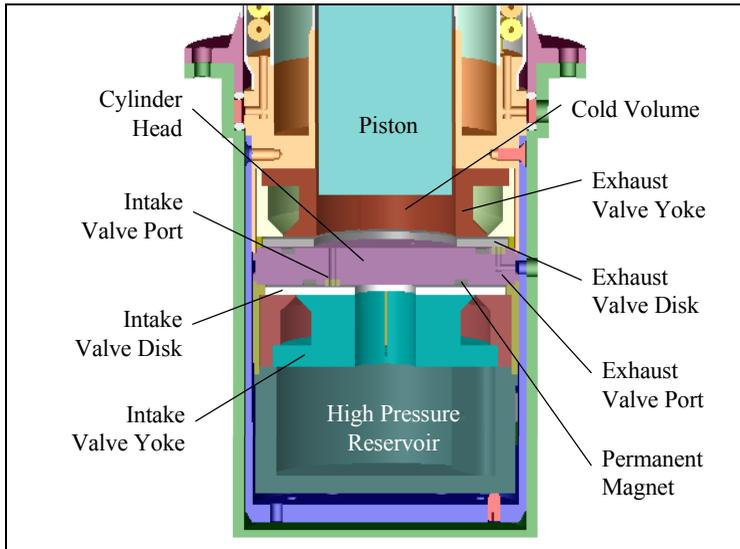
**FIGURE 3.** Electromagnetic *Smart Valve*
