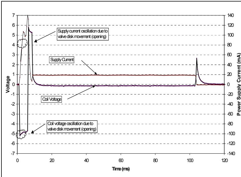
FIGURE 4. Smart Valve Shaped Voltage-Current Pulse
