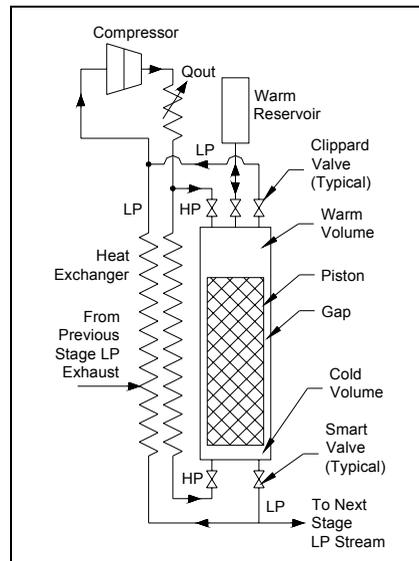
FIGURE 1. Floating Piston Expander
