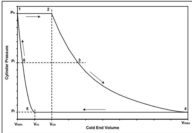
FIGURE 5. Ideal Cycle P-V Diagram
