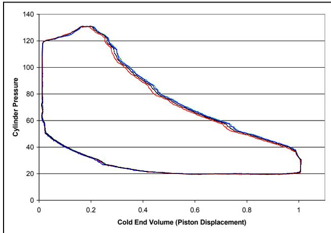
**FIGURE 7.** Four-Reservoir Multi-Cycle P-V Diagram
