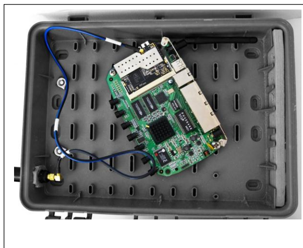
Figure 4. Netgear WGT634U router hardware shown within a typical roofnet weather-resistant environmental package to provide a size comparison. (Image by Lauren Keville used with permission of Kurt Keville of MIT Roofnet.)
