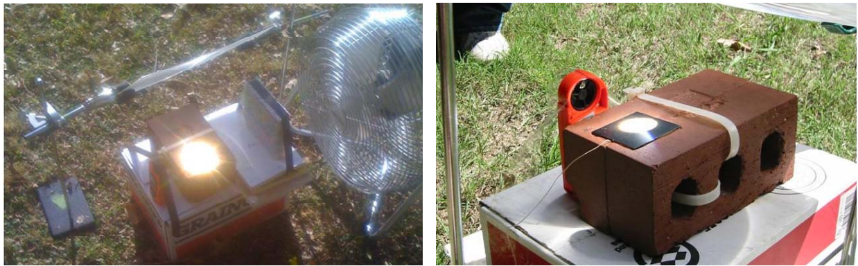
Figure 5. Small-Area Fresnel solar concentrator apparatus with the brass target unpainted (left) and painted black (right). These images show the marked difference in energy reflectance realized between these two surface treatments.
