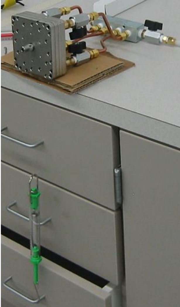
Figure 2: Simple Tesla turbine static torque measurement configuration showing spring gauge alignment.
